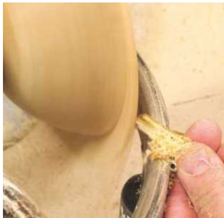
▲ Pic.23 As the piece gets thinner, having too much bevel in contact with the wood will become a problem. Using the smaller bowl gouge in a pull cut will put less pressure on the surface and cause less vibration
